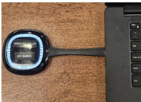
**Step 2:** The lights on the dongle will flash. Wait until the lights remain solid then press down on the dongle (it's a big button).
